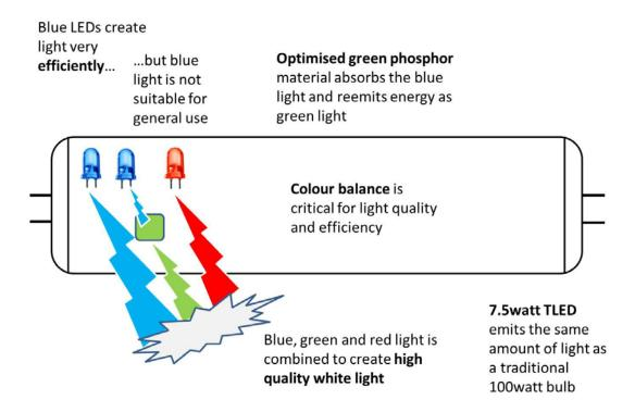
At the heart of this TLED is Philips Lumileds InGaN LED, recognized as the world's highest performing blue LED. This LED significantly boosts efficiency from the earlier generation which was at the heart of the L Prize (see below) winning replacement 60W bulb.
