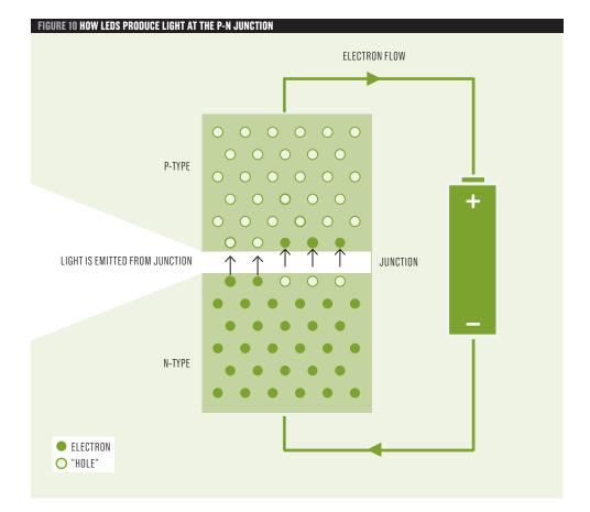
The light that LEDs produces comes from surplus electrons that race energetically towards quantum holes across the border in a sandwich of two different semi-conductor materials. One material is a N (negative) semiconductor, usually silicon, which has too many electrons due to the makeup of a special impurity in its lattice. The other is a P (positive) semiconductor that has too few electrons due to the special makeup of a different impurity, thus creating "holes" in its lattice.
