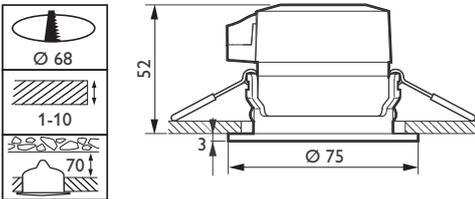
Abmessungen in mm
