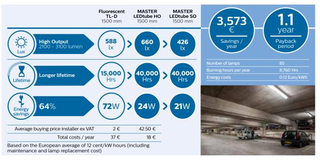
> Choose High Output LEDtubes for high light output with the best lm/w
