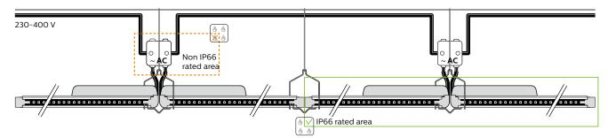
The "none IP rated area", must be build into an >IP66 environment. E.g. into a water tight junction box or water tight connectors.
