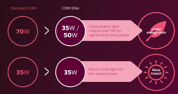
Switch both lamps and drivers to lower wattage versions and you can make significant energy savings. In cases of tight budgets, this is a good alternative to buying completely new luminaires as it requires a smaller initial investment.
