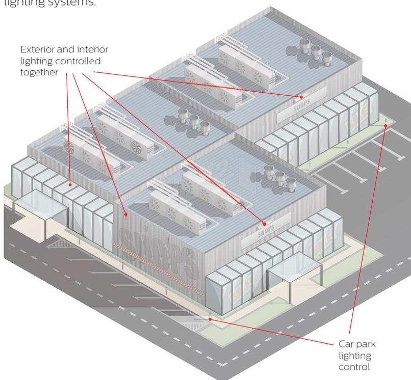
Supporting DALI protocols, EnvisionManager can complete mandatory DALI emergency lighting testing, visualize energy usage via Dashboard and monitor system component health, to streamline ballast replacement and manage relamping schedules.
