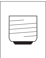
E40 DIN: 49625 IEC: 7004-24 ANSI: Mogul screw base C 81-10-1976 sheet 1-17-1
