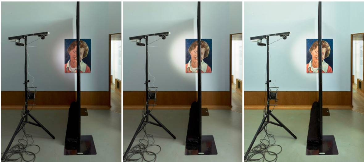
Test installation with artificial light on the left and daylight on the right. Left: Halogen spotlight without fluorescent ambient light: red haze. Center: Philips StyliD PerfectBeam Variable Spot without fluorescent ambient light: too much emphasis on the lighting. Right: Philips StyliD PerfectBeam Variable Spot in combination with fluorescent ambient light: the best effect.
