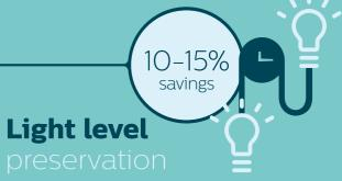
Over time, the brilliance of the LED luminaires decreases due to a natural ageing effect, which is why the lights are always 'over-specified' to compensate for lumen depreciation. By dimming lights at the beginning of their lifetime and gradually increasing their power output, you can ensure a uniform level of light in a store. As well as creating a consistency in the customer experience, it's possible to make significant savings in energy over time.
