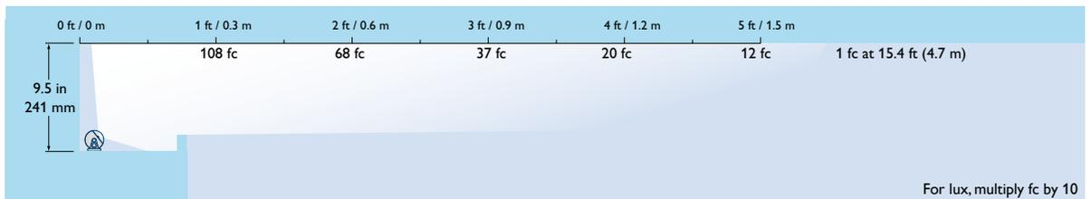
As the diagram above shows, properly aiming fixtures let you achieve dramatic and unusual effects from coves. Here, eW Cove MX Powercore fixtures are rotated in such a way as to create a grazing effect on the ceiling, throwing bright white light to a distance of over 5 ft (1.5 m) toward the center of the room from a perimeter cove.
