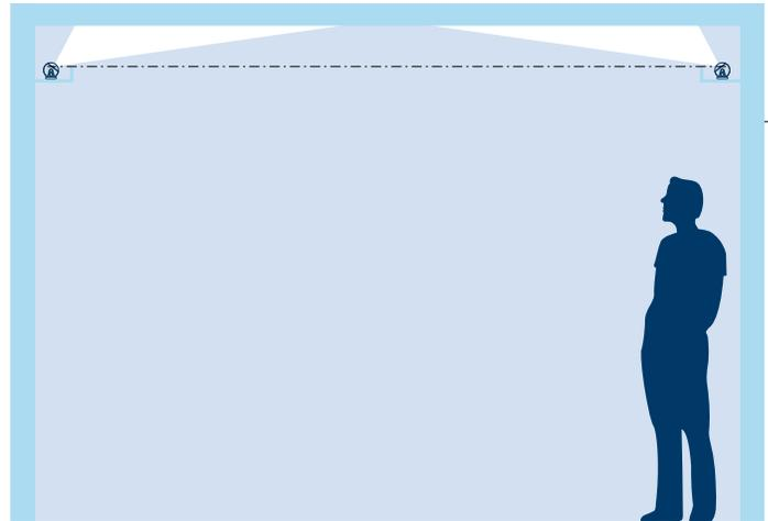
**For coves less than 9 ft (2.7 m) from the floor,** determine the line of sight by drawing a horizontal line from the top edge of the cove fascia to the back of the cove.
