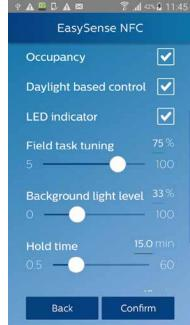
EasyAir parameters can be configured via Philips field apps. Two versions are available:
