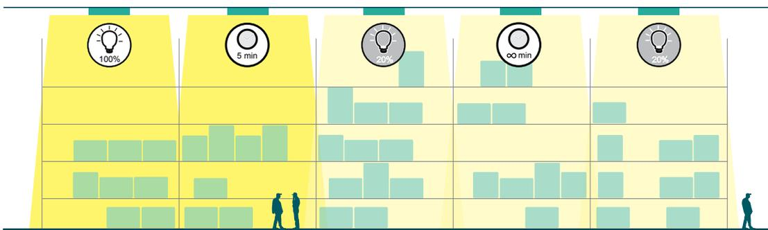
Traditionally, some spaces in a manufacturing facility are configured to stay on all the time, wasting a significant amount of energy. With SpaceWise Technology it is possible to reduce this energy waste by dimming the lights to a background level during unoccupied periods.
