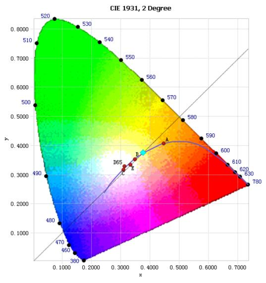
Tristimulus values(x, y): (0.3764, 0.3761) Chart 2: Chromaticity Diagram per Sphere - Spectroradiometer Method
