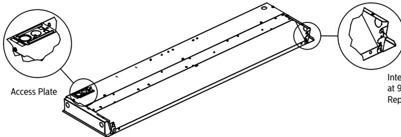
Integral Grid Clips – Bend upper tab outward at 90°. Bend lower tab outward approx. 20°. Repeat for all four corners.
