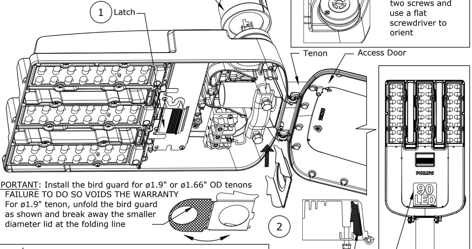
To change the orientation of the socket, loosen the two screws and use a flat screwdriver to orient
