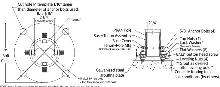
NOTE: Internal clearance of tenon/pole mounting bolts dictates allowable area for stub-ups.
