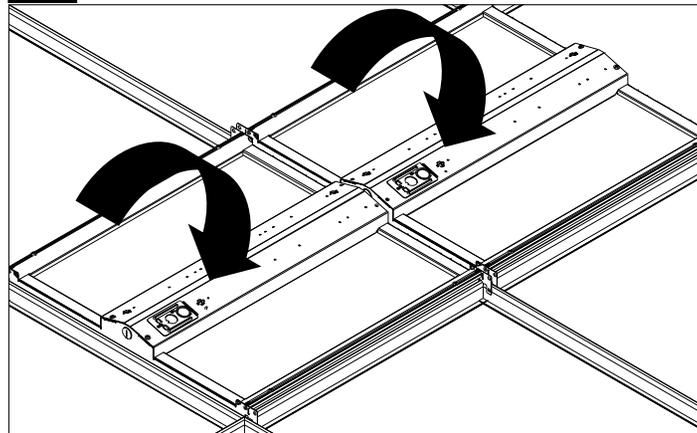
Attach the low voltage driver wires using the quick connect terminals. Install the driver while ensuring that all wires are covered and free from binding. Retain the covers by re-using the screws that were removed.
