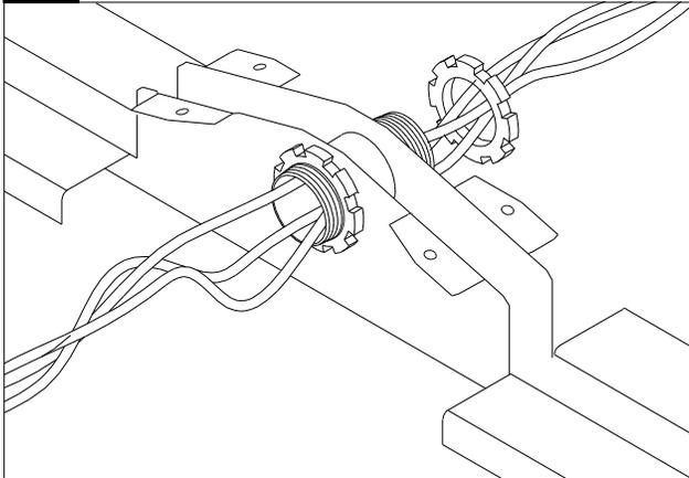
Feed the wires through the nipple and make all the electrical connections between the fixtures following the correct wiring color code.
