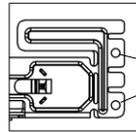
Holes to secure by nail or by screw
