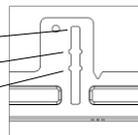
Mounting system is designed to install into channel with a height dimension of  $\frac{1}{2}$ " ,  $\frac{7}{8}$ " or  $1\frac{1}{2}$ ".
