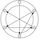
Use several rotations of the following sequence to tighten the lens ring screws, to 25 in/lbs. Mount Fixture as high above grade as possible to prevent debris and water standing on fixture surface.
