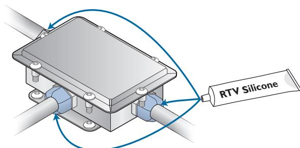
**⚠** For wet or damp locations seal all points of entry to prevent water infiltration. Use RTV Silicone and weatherproof junction boxes.
