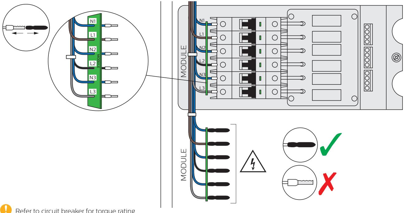
! Refer to circuit breaker for torque rating
