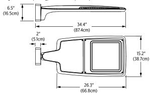
Slip fitter **(SF)**Weight: 32 Lbs (14.6 Kg) EPA: 0.38ft<sup>2</sup> (.035m<sup>2</sup>)
