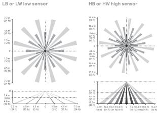
Note: The beam patterns shown are intended solely as a general guide and are not to scale. Sensing capabilities and coverage area depend on many factors including the size, speed and direction of travel of persons and vehicles; sensor mounting height; environmental and site conditions; etc.
