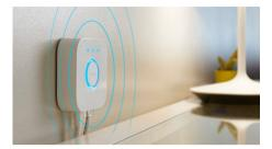
Connect your Philips Hue lights with the bridge to control your lights from your smart phone or tablet via the Philips Hue app.
