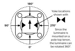
Note: The hand hole will normally be located on the pole at the 0° point.
