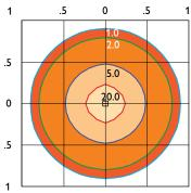
LPF3 85W - 20' Mounting Height, 0° Tilt Mounting Height 30 25 20 15 10 Multiplier 0.44 0.64 1.0 1.8
