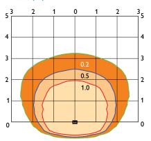
Notes: Grid is in multiples of mounting height and values shown are in footcandles. Values shown are based on initial lumens.
