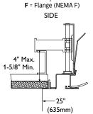
(NEMA Type F) Flange for acoustical ceilings using concealed mechanical suspension. Swing-jack mounting brackets: adjustment 4" max.and 1-5/8" min. Refer to sheet 801-CL for cut-out information.
