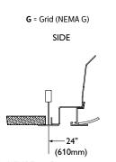
(NEMA Type G) Lay-in acoustical ceilings using exposed grid suspension, with tees for luminaires on 24" x 48" spacing.
