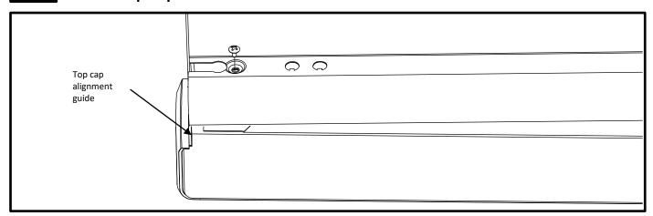
Tuck wires into fixture then replace top caps and secure with screws provided with either a Robertson #2 screwdriver or a Phillips screwdriver.
