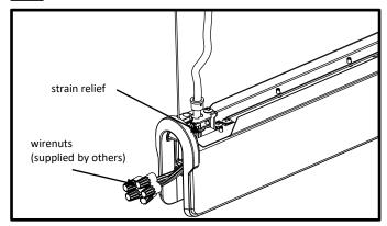
NON-POWER LOCATIONS: Cap all wires and tuck into wire cavity.
