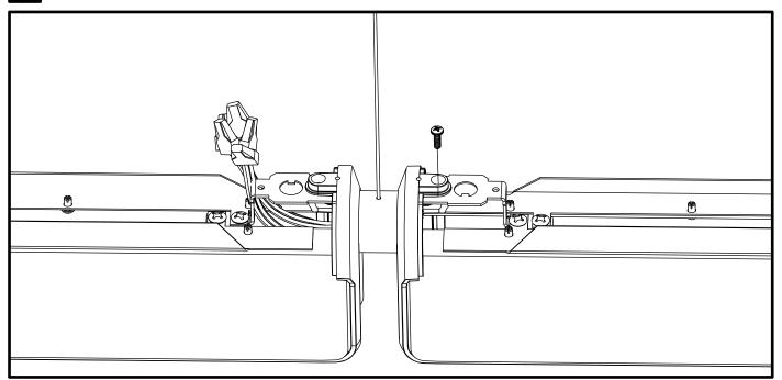
Feed wires from second fixture through the straight joint. Secure with screw provided in joint kit with a Phillips screw driver. Make power connections with supplied quick-wire connectors.
