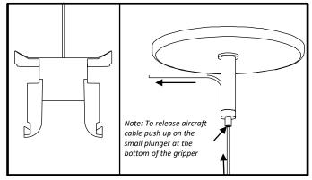
Insert aircraft cable through the joints and mount them in appropriate locations as supplied by layout drawing.
