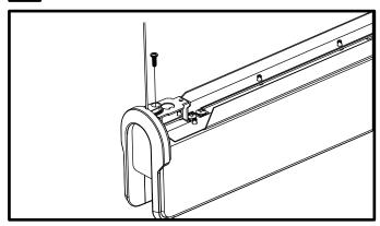
Secure endcaps with screw provided with a Phillips screw driver.
