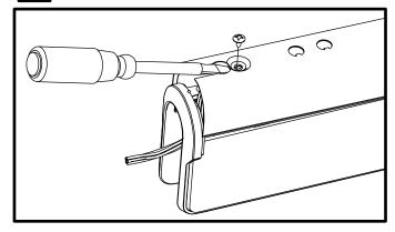
Remove screws along top of fixture with a Phillips or Robertson screwdriver and remove the top cap with the help of a flat head screw driver.
