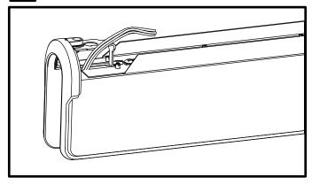
Feed wires into the fixture on both ends of the fixture. Do this for all fixtures on joining ends.
