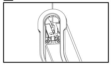
Insert aircraft cable into diecast cross plate.
