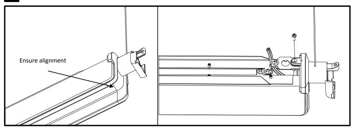
Mount the fixture to the continuous run joint. *Ensure continuous run joint is seated properly in the fixture*. Secure with screw provided in joint kit with a Phillips screw driver.
