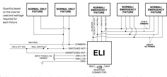
Total dimmable power based on the inverter used and power requirements of each fixture
