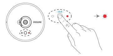
Make sure the sensor successfully detects movement within the designated area, especially at the perimeter and entry points.
