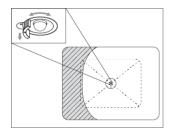
Performing a walk test will help optimize the occupancy detection coverage and sensitivity. Commission the sensor before you perform the test.
