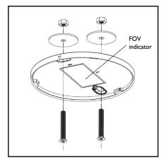
Refer to the rectangular symbol on mounting plate for FOV orientation.
