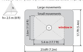
Larger areas will require multiple sensors. The retractable sensor shield can be rotated to partially mask the sensor's field of view and prevent unwanted movement detection.
