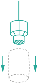
4 Remove the existing cover by lowering it over the main housing
