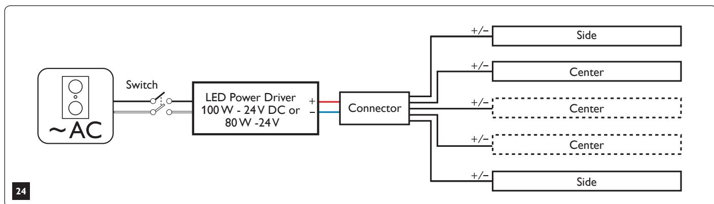
To allow for variance in the installation, it is not recommended to load the power driver beyond 90% of its rated maximum power.
