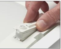
Step 2: Remove the two wires that were secured to the back of the plate and insert them in an approved sensor for use with EvoKit. They are not polarity sensitive.
