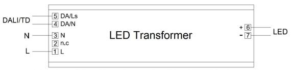
For independent application: minimum wire cross section = 0.75mm<sup>2</sup> / 18AWG for output current > 2A
