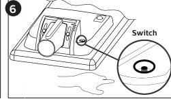
To switch ON the luminaire press the switch button shown in below figure.
