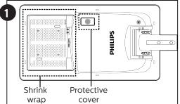
Remove shrink wrap and protective cover before installation.
