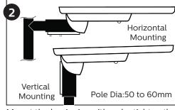
Mount the luminaire with pole, tighten the bolts with torque of 8 Nm.
