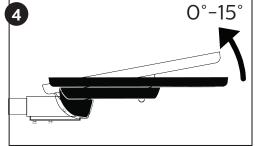
For tilt mounting to suit various geography, luminaire can be tilt mounted from 0 to 15 deg
