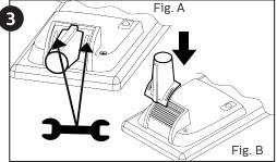
For vertical mounting unscrew and remove pole mounting bracket and assemble it as shown in Fig. B.
