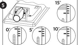
For accurate angle positioning, match pole marks mounting piece marking with luminaire marking
