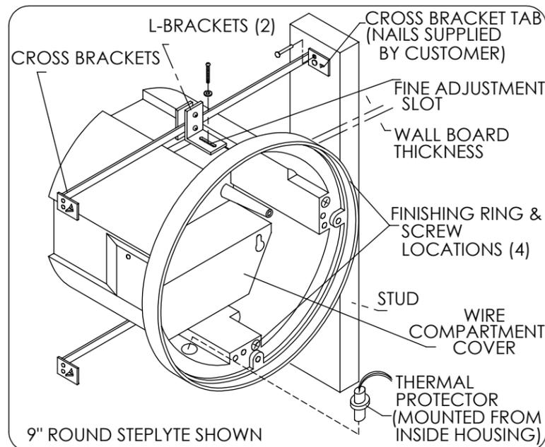
1. Using the template supplied, cut a level hole through the wall board to fit around the fixture housing. Failure to level hole will cause the fixture to have a tilted appearance.
