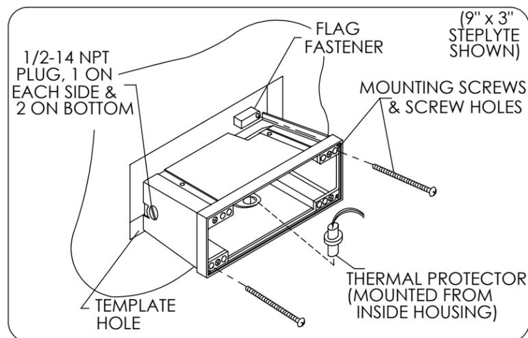
1. Using the template supplied, cut a level hole through the existing wall between existing studs. Failure to level hole will cause the fixture to have a tilted appearance.
