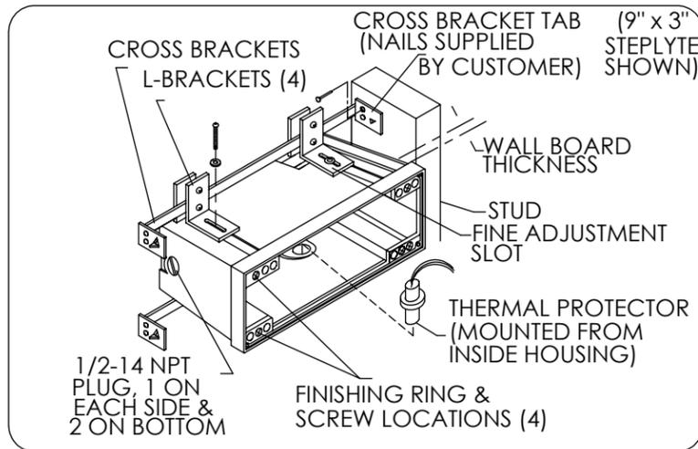
1. Using the template supplied, cut a level hole through the wall board to fit around the fixture housing. Failure to level hole will cause the fixture to have a tilted appearance.
