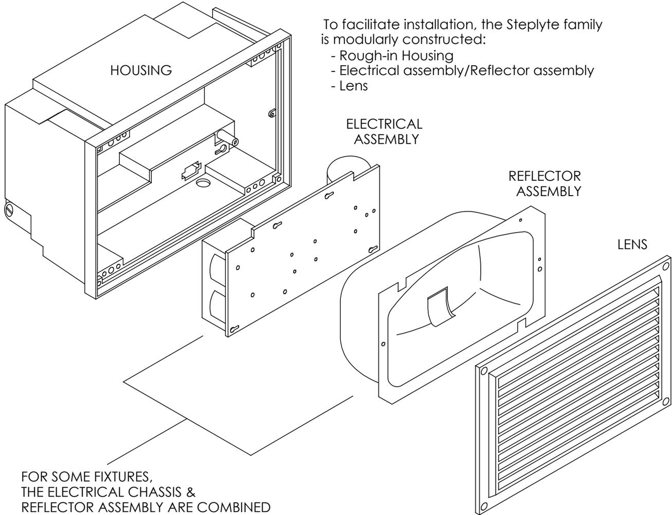
To facilitate installation, the Steplyte family is modularly constructed:
