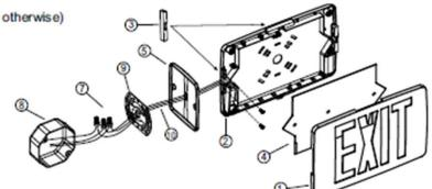
**NOTE:** This fixture is for use only with 3-1/2" octagon, 4" octagon, 4" square or single-gang junction boxes, on an unswitched circuit. See Wiring Diagrams and "To Remove Directional Indicators" below before beginning fixture installation. **On fixtures with battery:** Connect battery only after continuous power can be supplied to fixture. Allow 24 hours before initial test or for full charge.
