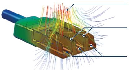
Airflow driven by natural convection from the temperature difference between the upper and lower zones efficiently draws heat away.
