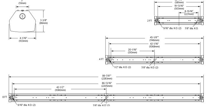
\*For integral controls option, overall length is 1-3/8" (35mm) longer.
