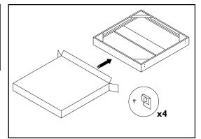
Remove fixture from packaging and locate hardware. Leave spacers in place for install.
