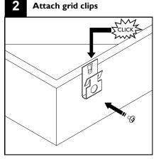
Attach grid clips to fixture using supplied screws.
