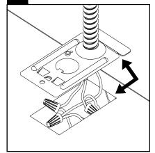
Remove pre-installed wire access plate Connect power feed to the leads provided Note: A second wire knockout is provided for daisy-chain wiring additional fixtures
