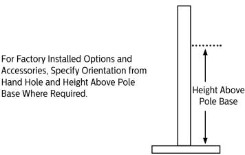
Orientation is measured clockwise from the Hand Hole Center.
