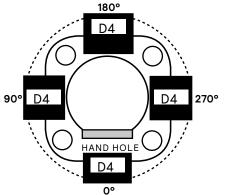
D4 Drilled for 4 Luminaires at 90°
