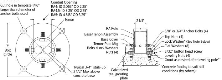
NOTE: Internal clearance of tenon/pole mounting bolts dictates allowable area for stub-ups.
