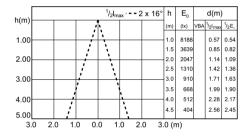
Beam diagram - MC CDM-R Elite 35W/930 E27 PAR3OL 30D
