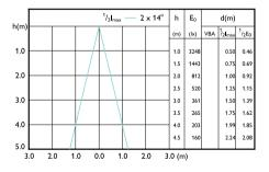
Beam diagram - MAS LEDspot D 12-100W E27 927 PAR30S 25D Beam diagram - MAS LEDspot D 13-100W E27 927 PAR38 25D
