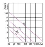
Accent Diagram - MAS LEDspot D 13-100W E27 927 PAR38 25D Accent Diagram - MAS LEDspot D 12-100W E27 927 PAR30S 25D
