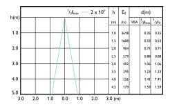
Beam diagram - MAS LEDspot D 12-100W E27 927 PAR30S 25D Beam diagram - MAS LEDspot D 13-100W E27 927 PAR38 25D Beam diagram - LEDClassic 10-80WPAR38 827 25D 1CT/3 SRT
