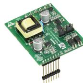
**DGBM200 2 Channel Signal dimmer driver module**
