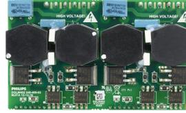
DGRM204 2 x 4 A Relay control module
