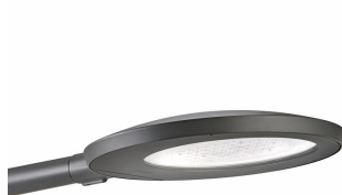
CitySoul gen2 Large - LED module 12000 lm - 830 warm white - Power supply unit with DALI interface - Safety class II - Distribution medium 50 - Clear glass - Gray - Philips standard surge protection level - - - Side-entry for diameter 60 mm
