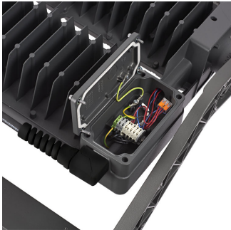
Electrical Connection box of BVP527 floodlight with cable gland and push-in terminals enabling electrical connection to driver box (Grey painted housing)
