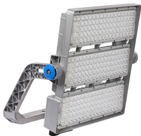
ARENAVISION LED GEN3 LARGE - LED module 180000 lm - 957 cool white - Power supply unit with DALI interface - Symmetrical
