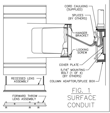
NOTE: COLUMN ADAPTOR/SPLICE BOX IS SECURED TO COLUMN WITH 5/16" BOLTS (BY OTHERS). STRUCTURAL MEMBERS MUST BE PRESENT IN COLUMN TO ACCEPT BOLTS.
