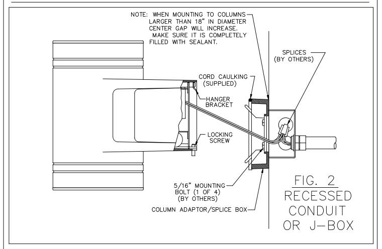
TO REST AGAINST ADAPTOR. REPLACE LOCKING SCREWS INSTALLED IN LUMINAIRE WITH LOCKING SCREWS SUPPLIED WITH ADAPTOR AND TIGHTEN. REMOVE EXCESS CAULKING.
