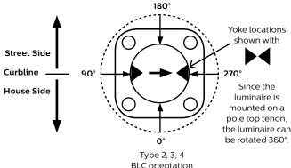
Note: The hand hole will normally be located on the pole at the 0° point.
