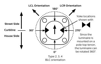
Note: The hand hole will normally be located on the pole at the 0° point.
